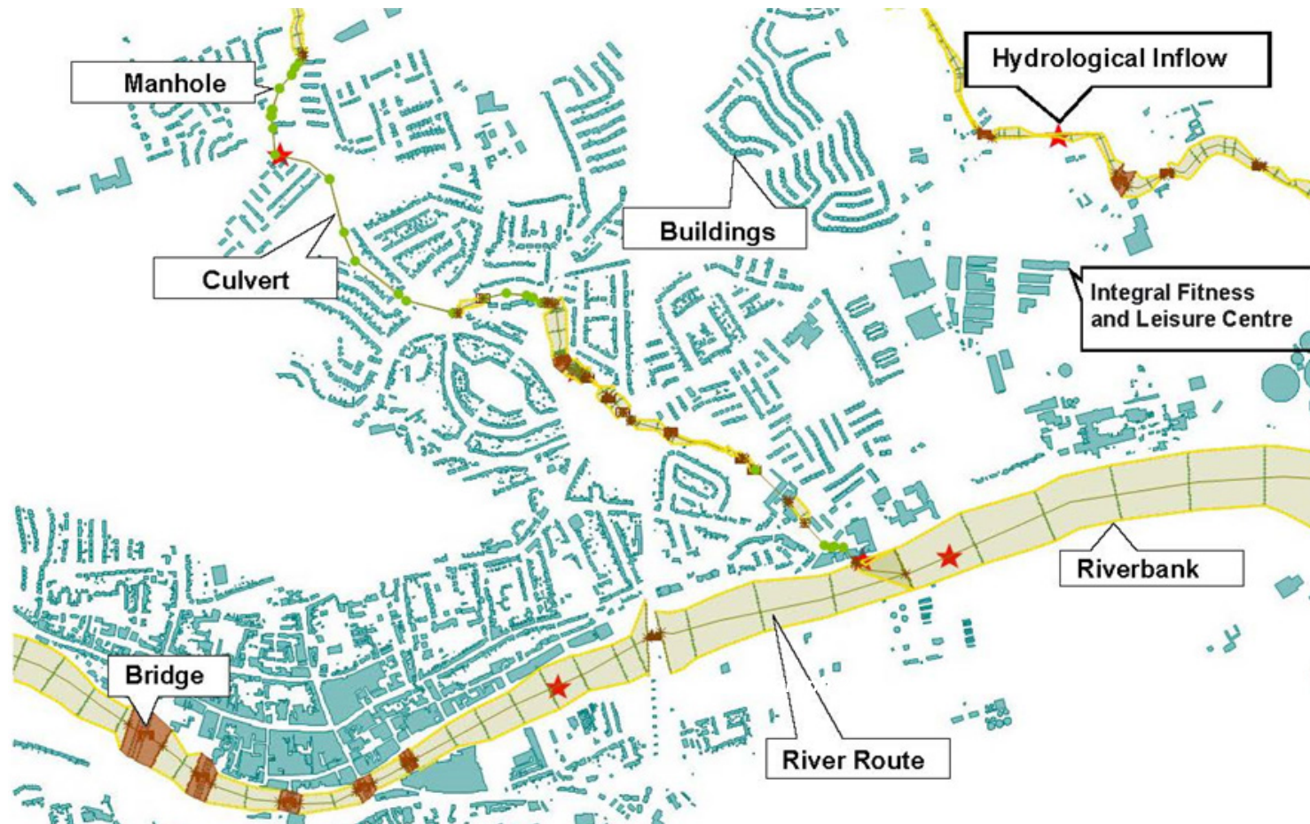
The image shows an extract from the computational model which has been constructed to allow simulation of a range of flood events and to assess possible flood relief measures.
