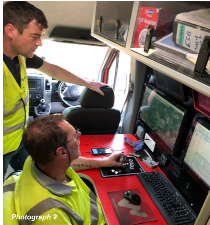
Photograph 1 is showing the survey contractor getting the equipment ready for the survey. Photograph 2 is showing the survey contractor conducting the CCTV survey of the culverts.
